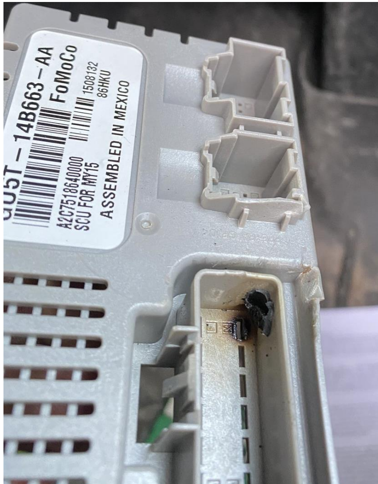
Figure 8 - SCME Damage from Terminal Failure
