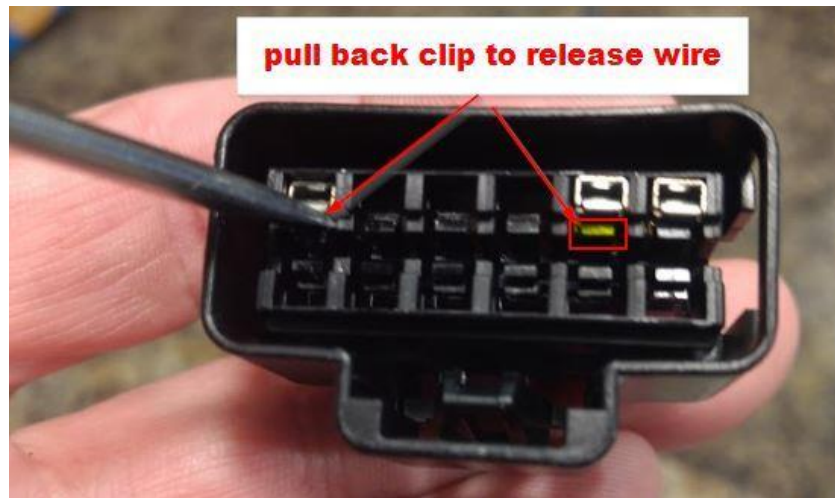
Figure 19 - Terminal Unseating Channel and Release
