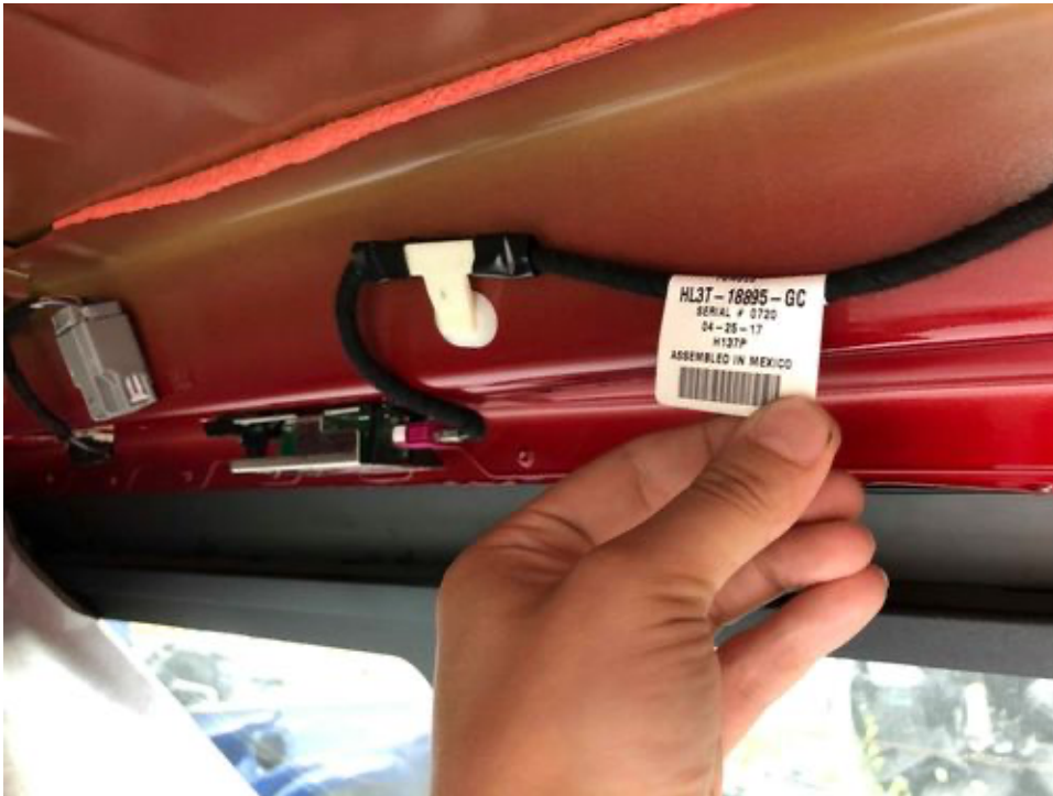
PIFA Antenna Location and GSM Antenna Cable
